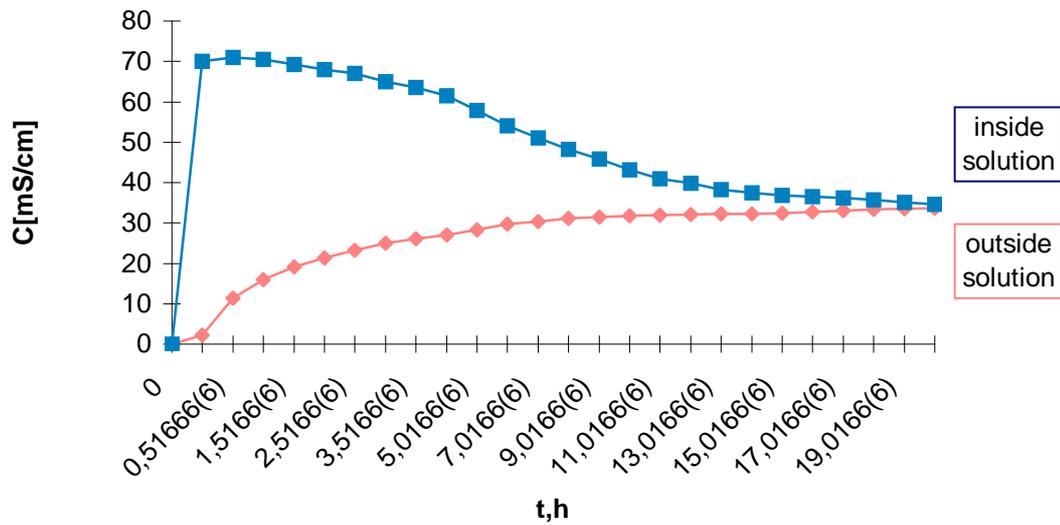
**Figure 4: Variation of the conductivity with time when dissolving 100 ml 12% solution of FeCl<sub>3</sub> in 300 ml distilled water through a polycarbonate membrane ( $d_o = 0,4 \mu\text{m}$ ;  $S = 7,5 \text{ cm}^2$ )**
