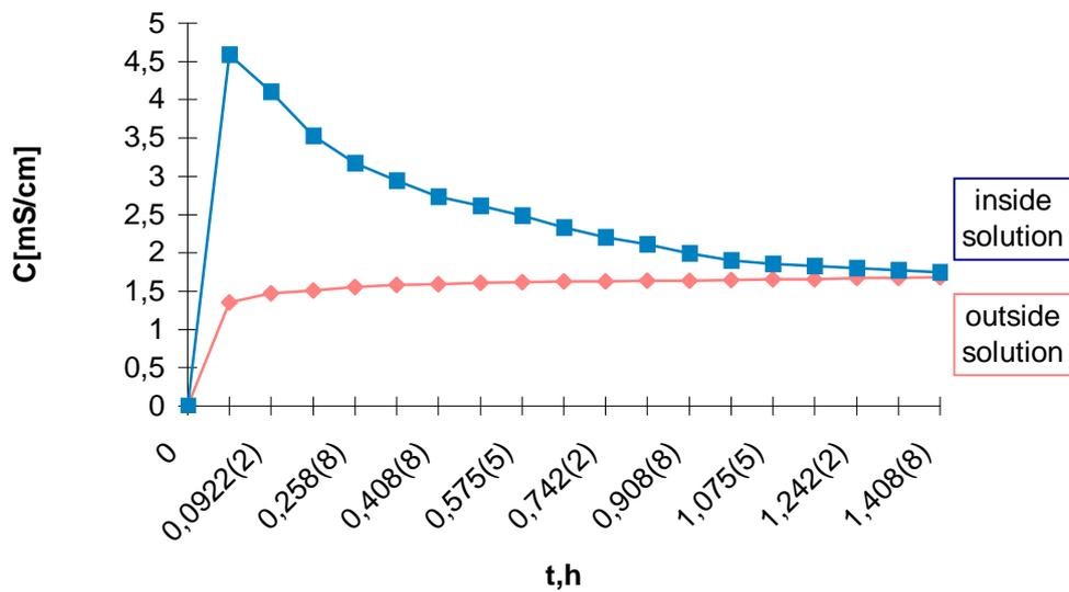
**Figure 5: Variation of the conductivity with time when dissolving 100 ml 25% solution of FeCl<sub>3</sub> in 300 ml distilled water through a polycarbonate membrane ( $d_o = 8 \mu\text{m}$ ;  $S = 7,5 \text{ cm}^2$ )**
