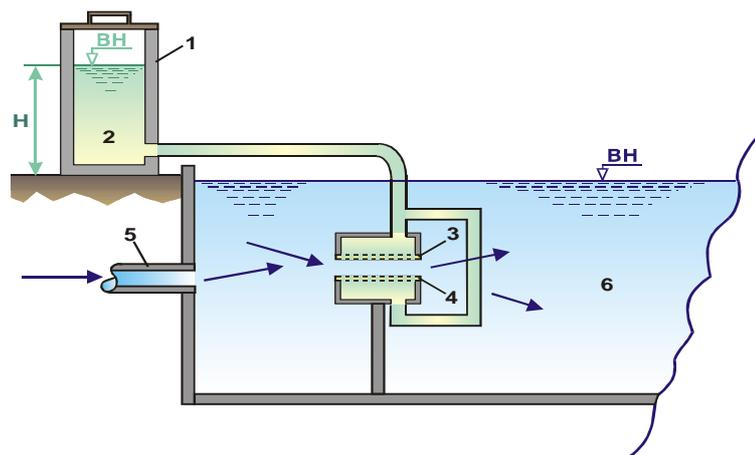
**Figure 7: Dynamic dosing membrane device /with head pressure in the reagent container/ - 1 – reagent container; 2 – chemical reagent; 3,4 – membranes; 5 –inflow; 6 – reaction basin**
