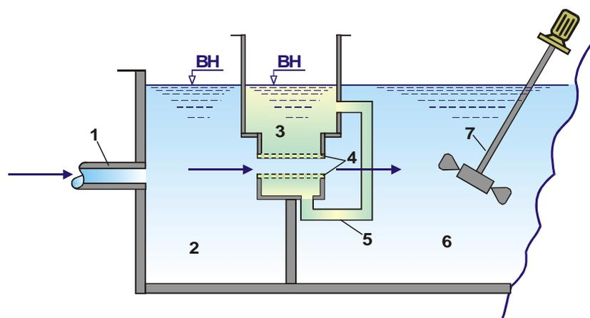
**Figure 8: Dynamic mambrane dosator /witout pressure in the reagent container/ - 1 – inflow; 2 – entrance basin; 3 – reagent container; 4 – membranes; 5 – conecting pipe; 6 – reaction basin; 7 - mixer**
