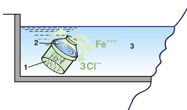
**Figure 6: Model scheme of a dosing device /a single canister, which can be used in sudden pollutions, for precipitation, neutralizations etc./ - 1 – solution of  $FeCl_3$ ; 2 – membrane; 3 – reaction basin**
