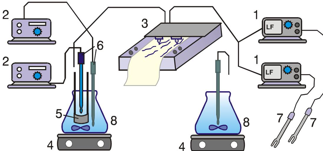
**Figure 3: Experimental device-** 1-conductivity meter; 2- pH-meters; 3- recorder; 4 – stirrers; 5- membranes; 6,7 – electrodes; 8-erlenmayer flask
